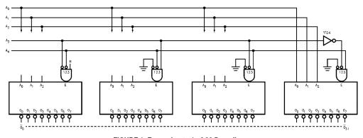
FIGURE 1. Expansion to 1-of-32 Decoding
